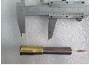
Figure 2. Configuration of joint made by EMF method.
